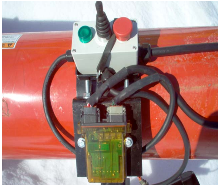
Picture showing proper mounting of motor mount- 15- 20" from intake of hopper
