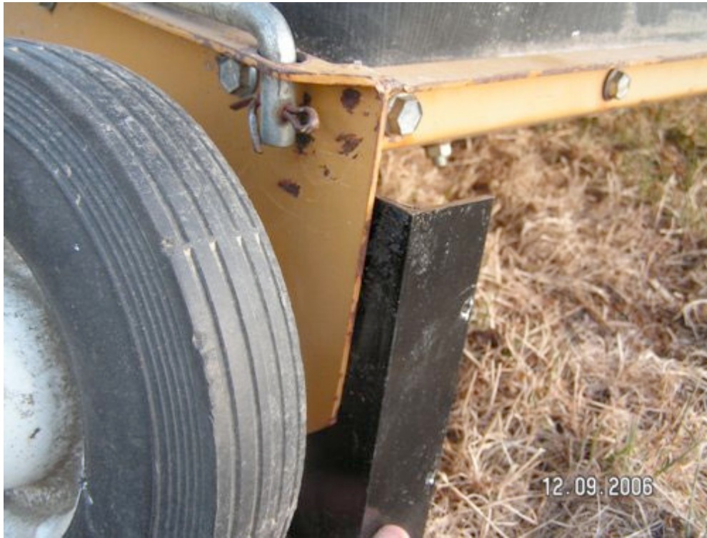
Outside mounting of angle iron bracket-- pushed out ward about 1/2"
