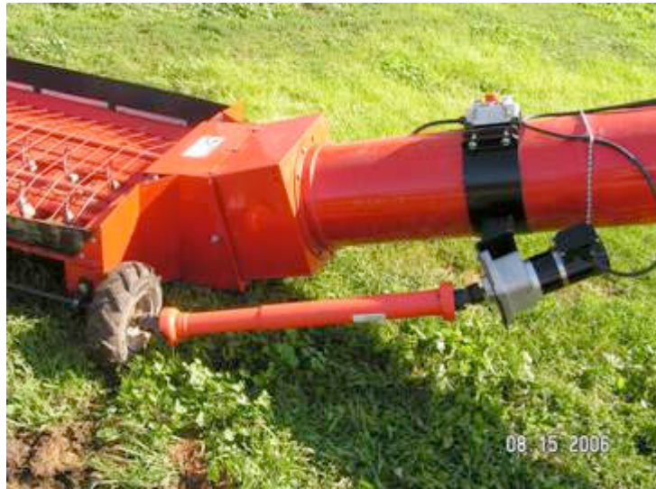
Complete motor and driveshaft and shield installed
