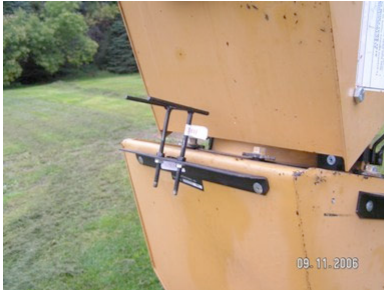
Proper mounting of the front bracket for the limit stops.
