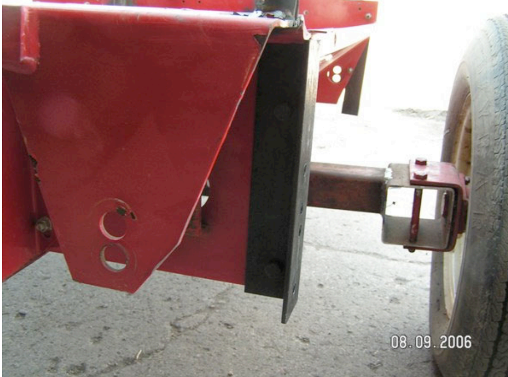
Picture showing the outside 10" angle iron mounted to hopper with 2 3/8"x 1" bolts and nuts.
