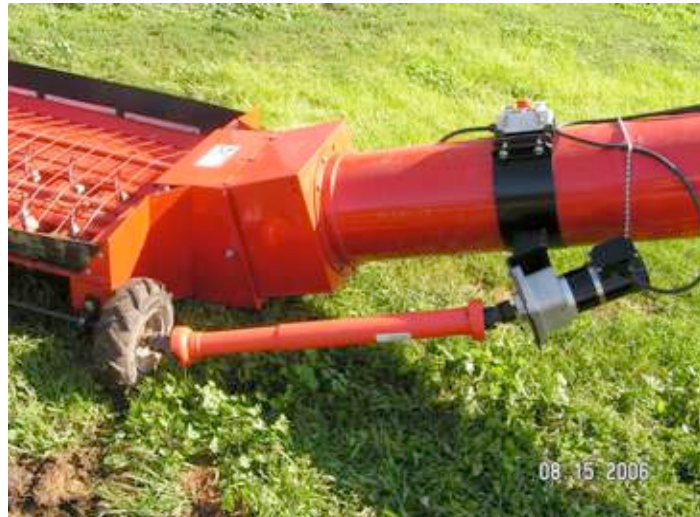
Complete motor and driveshaft and shield installed
