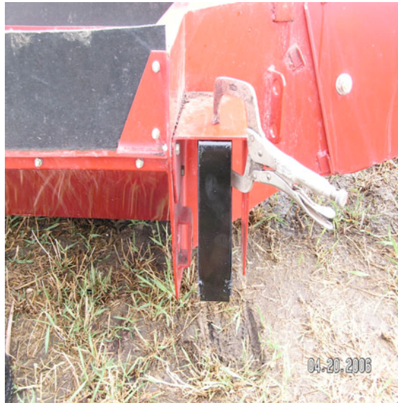
Picture showing mount for inside bearing support bolted to top of factory support.
