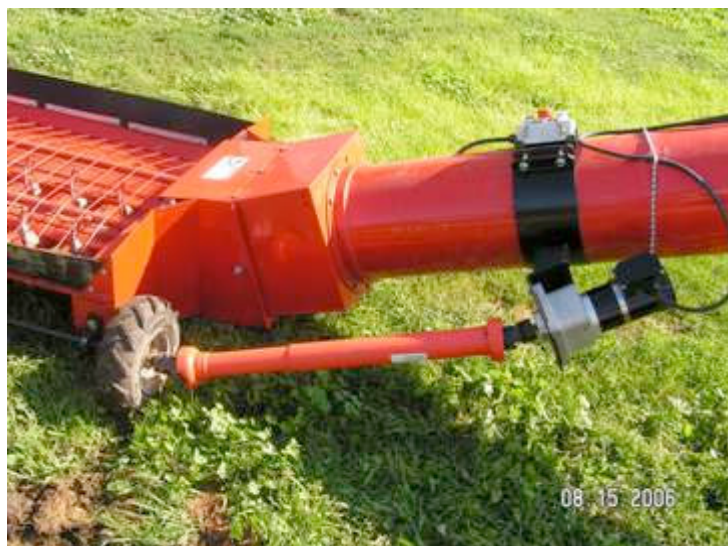
Complete motor and driveshaft and shield installed
