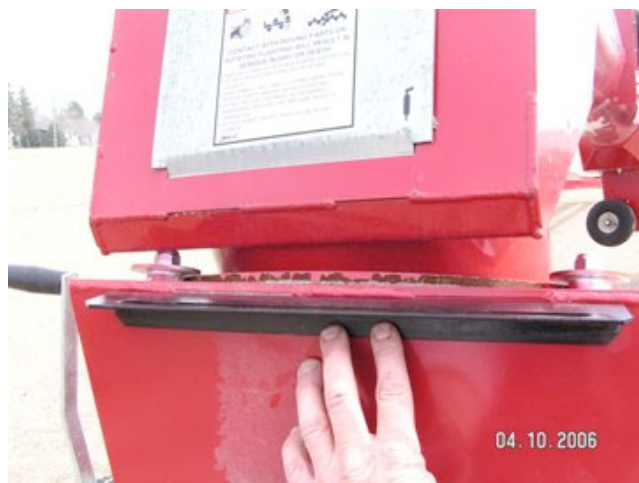
Picture showing proper placement of front mounting bracket parallel with auger boot and lowered approximately 1/4" below welding.
