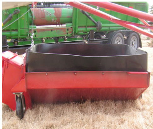
Typical 12" 3 wheeled hopper with the inside hopper wheels that swivel.
