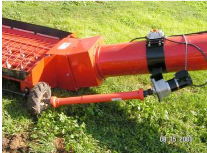
Complete motor and driveshaft and shield installed
