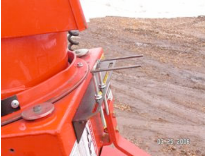
Proper position of the front stop with tabs facing away from auger boot.
