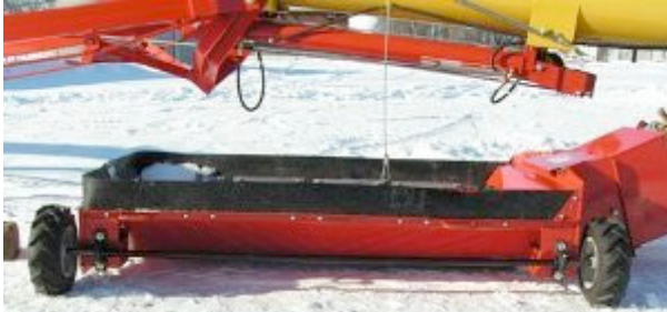
Picture showing hopper with axle, bearings and wheels installed.
