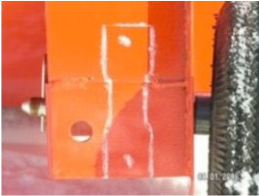
Picture showing where to place bearings if you have the factory mounting base.
