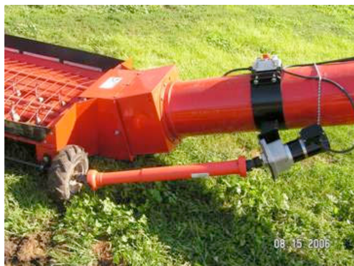
Complete motor and driveshaft and shield installed
