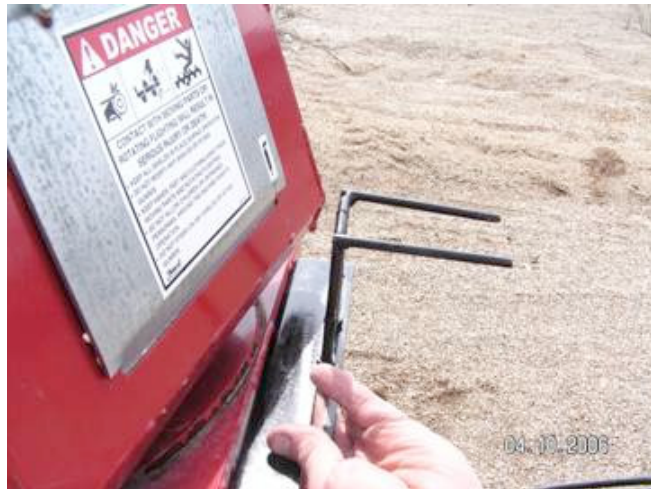
Picture showing front stop with stop tabs away from boot.
