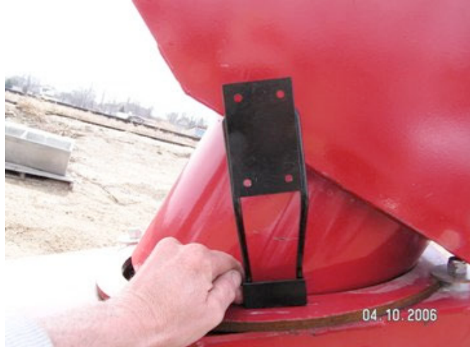
Picture showing side view of limit switch mounting.
