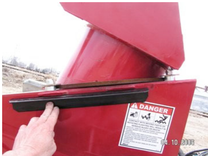
Picture showing proper position of side bracket on auger, 5"-6" from front of boot
