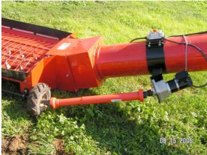
Complete motor and driveshaft and shield installed
